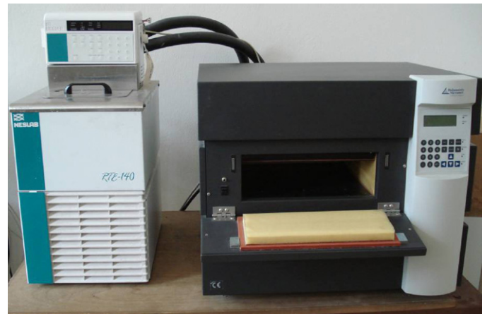
Fig. 5. Measuring device to determine thermal conductivity, Holometrix Lambda 2300.
